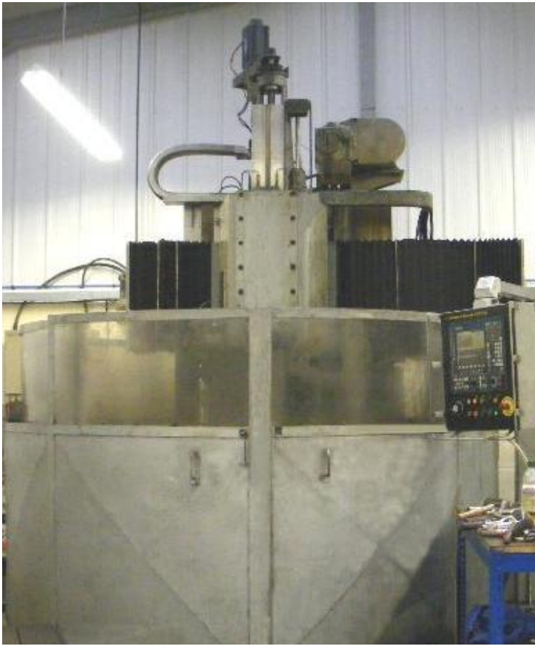
Above: Webster & Bennet 6ft CNC Vertical Turning & Boring Machine. Top right: A Bearing -Housing mounted on the Webster & Bennett turntable ready for initial machining, shown below this is a finished 500 mm Diameter Hub for a leading manufacturer of Mining Equipment after Turning and Boring operations.
