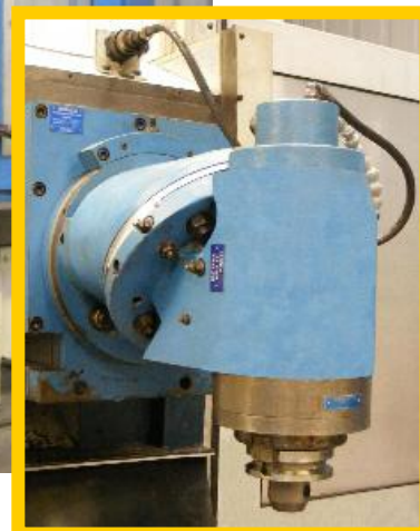
The Auerbach FBE 1500 fitted with a 360 degree rotary table and manually operated Universal Head (see inset left) provides Maple Worcester Ltd with a useful 4 + 1 Axis milling and drilling capability for components up to 1500mm x 900mm x 900mm in size.
